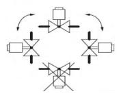
Metal shoe construction of the diaphragm allows for vertical installation, with less damage from debris and over pressure.
