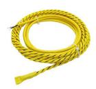
2-Core leak detection ropes include a 5FT lead wire, however this wire may be extended using 18-22 AWG. The total length of lead wire and sensing cable may not exceed 500FT. If more than 500FT is required, use multiple WLM controllers.
